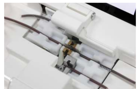
RF DOCKING Aligned welding with desired tubes
